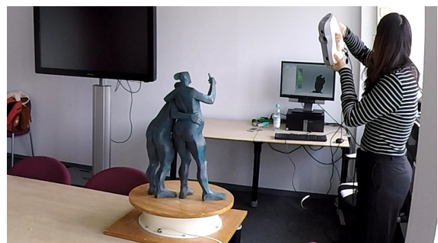
Figure 65. Set up of the 3D scanning.
