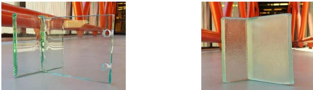
Fig. 1 Welded T-section (left) and fused T-section (right).
