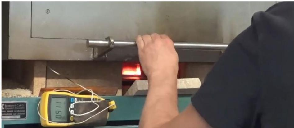
Fig. 5 Glass welding at second experiment, the web is being pressed on the flange.
