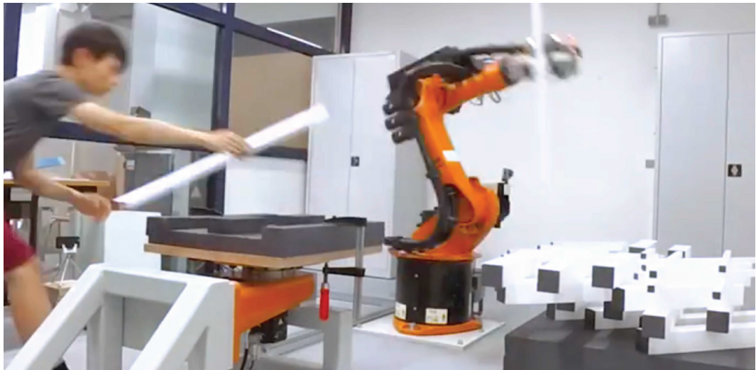
FIGURE 1 Human-robot collaboration during staking of linear components (© RB).
