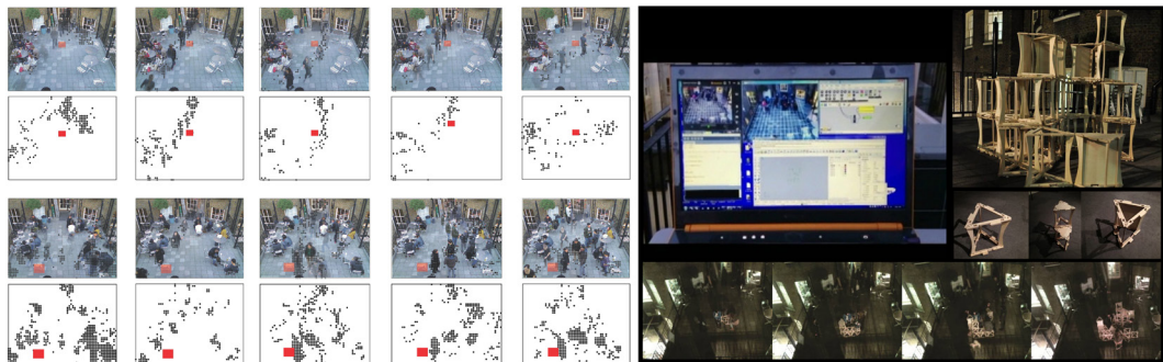
FIGURE 10 Snapshots of people monitoring as seen through the web cam and as analysed by blob-tracking algorithms.
