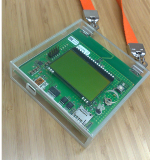
Figure 1.4: A custom made wearable sensor pack. This sensor pack is used in all studies presented in this thesis.
