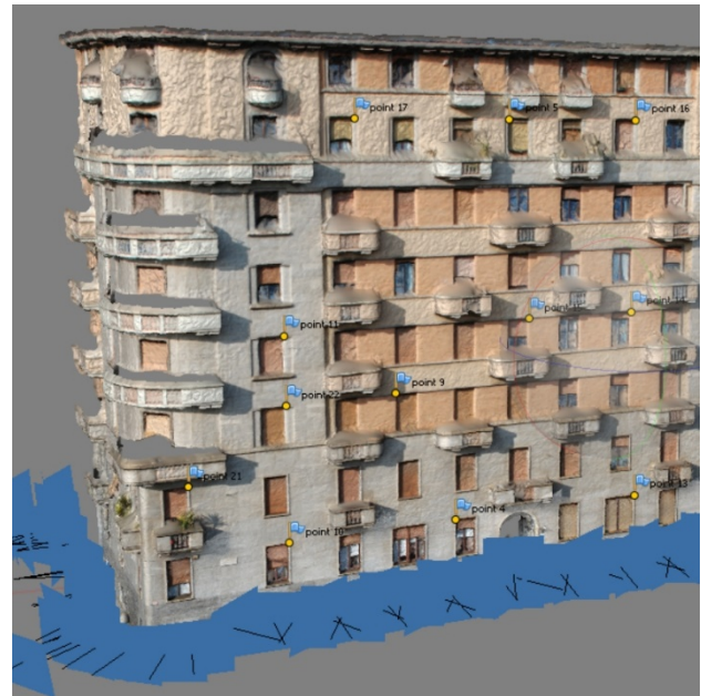
Figure 9 – Print-screen displaying the result of photogrammetric processing of RGB images in Case Study 2: the TIN model of the building façade textured with RGB photos, the location of extracted GCP's for co-registration of IR images, and estimated camera poses.
