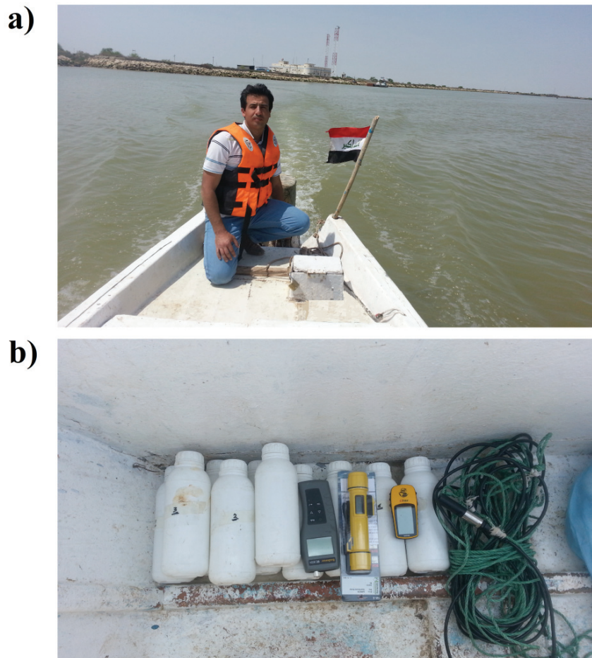
Figure 2-4. Boat measurement method; a) passing the military checkpoint and moving upstream keeping pace of the tidal wave during spring tide to the next measurement point, and b) water samples, conductivity meter, depth finder, GPS device and 10 meter cable.
