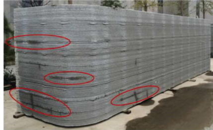
Figure 2.8: Signs of water-intake at the layer interface probably attributed to high interlayer porosity [39]
