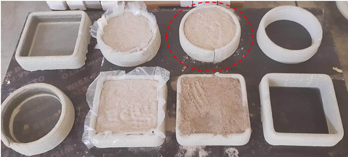
Figure 7.15: The specimens after t=14 days. The cracked specimen is highlighted in red
