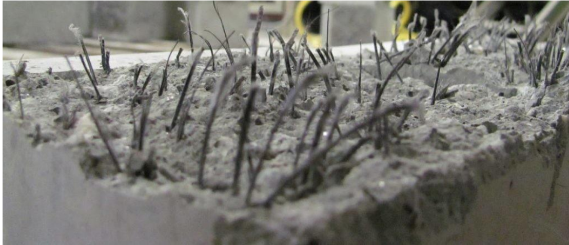
Figure 11: Fiber reinforced concrete after testing (Ataalla, 2018)
