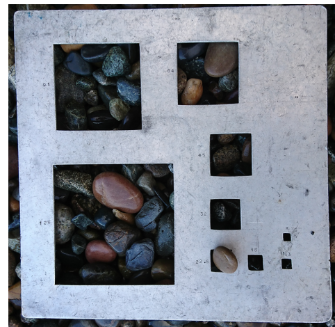
Figure B.1: Gravelometer used during the pebble counting on 06/11/2018.
