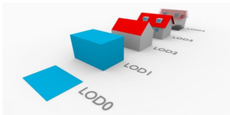
Figure 9. Levels of Detail in 3D City Models, from (Biljecki, Ledoux et al. 2014)
