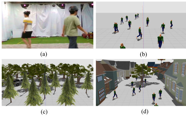
Fig. 8. Real-world scenario for velocity estimation test (a), and simulation worlds for mapping performance comparison (b)–(d). The pedestrian square world (b) contains only dynamic obstacles (the ground is excluded in the evaluation tests), while the forest world (c) contains only static obstacles. The pedestrian street world (d) contains both static obstacles and dynamic obstacles. (a) Velocity estimation test. (b) Pedestrian square. (c) Forest. (d) Pedestrian street.
