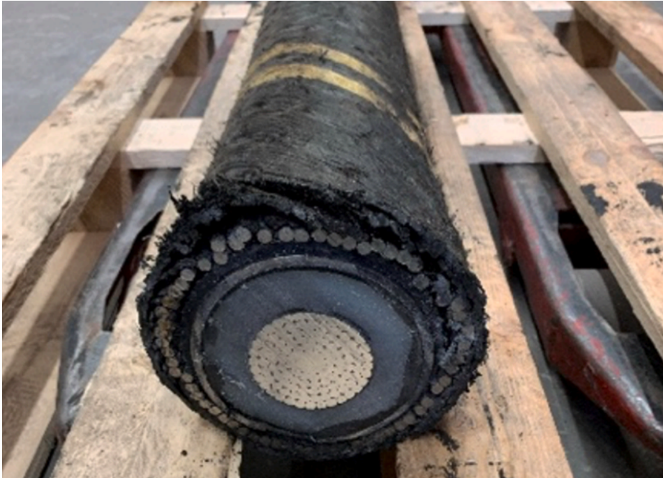
Figure 4.5: Subsea HVDC power cable tested by Ehlers et al. [11]
