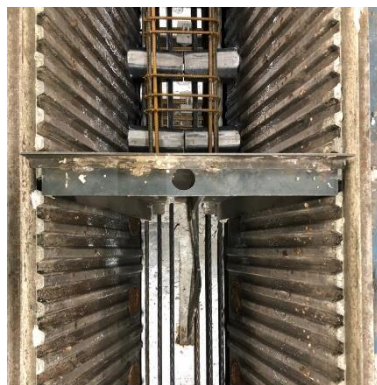
a) Tendons inside the molds
