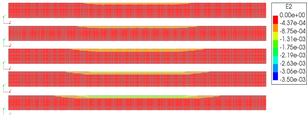
Figure 4.44. Minimum principal strains at 199, 222, 250, 276 and 345 kN
