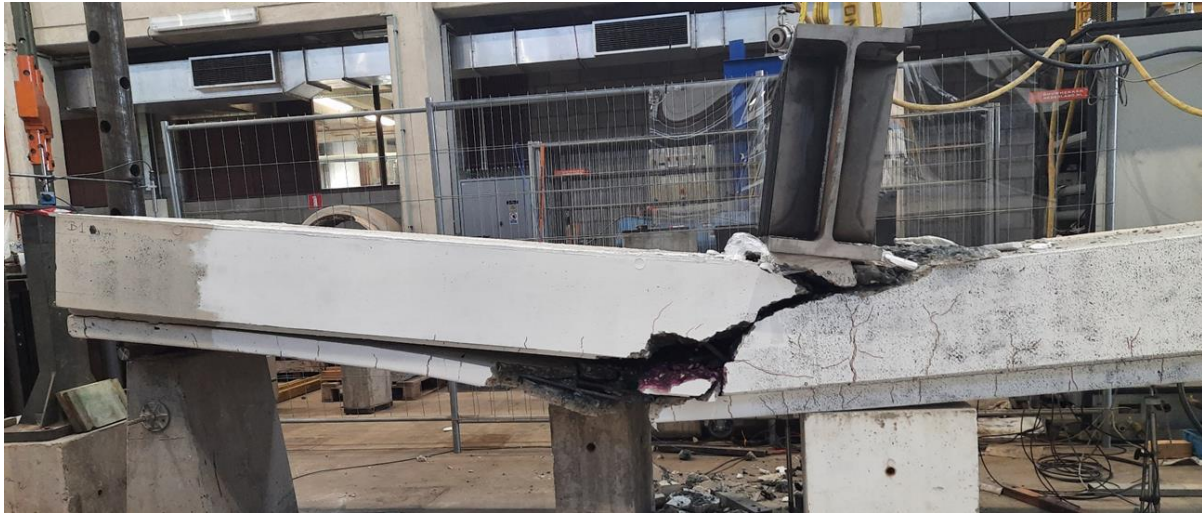
Figure 3.39. Failure of specimen subjected to flexural test after 9 months [61]
