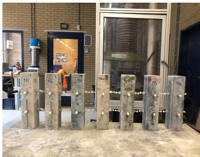
Figure 3.9. Elastic modulus testing
