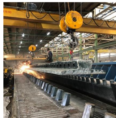
d) Cutting of tendons at the ends
