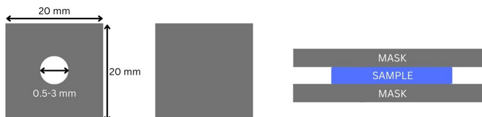
Figure 2.1: Schematic of stainless steel mask used for pattern etalon. The left mask is placed on top of the sample to create a pattern with a diameter ranging from 0.1-3 mm and the middle mask is the bottom mask used to securely hold the sample.
