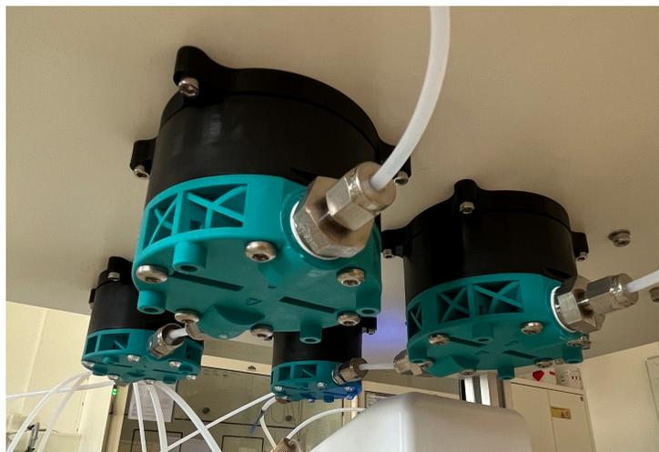
Figure 5.A.8: Pressure dampeners, screwed to the bottom of the BPR-setup.
