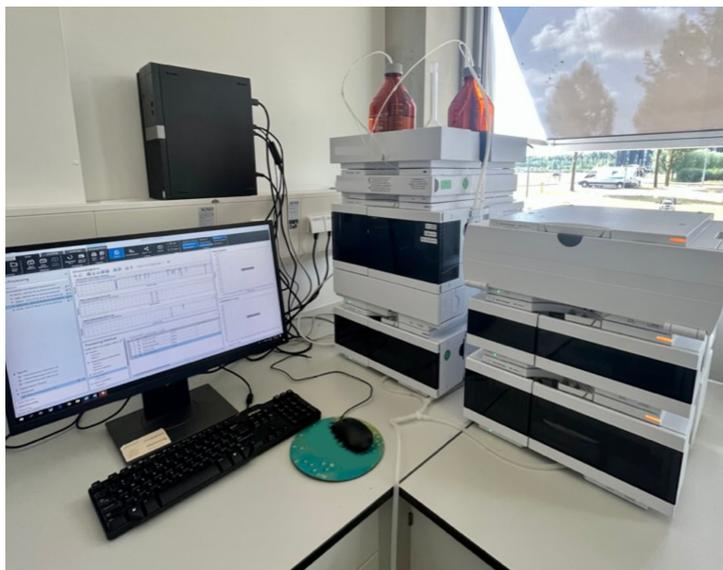
Figure 5.A.14: Agilent Technologies 1260 Infinity II HPLC setup.
