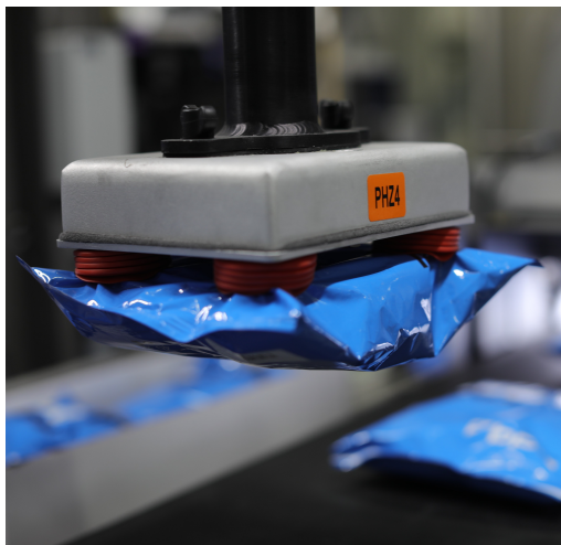
(A) Image of a standard suction cup based end effector
