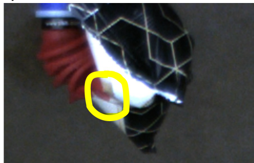
(C) In this frame the suction cup gripper has re-gripped the products. This is remarkable because the product has continued to move in the direction that originally caused the leak. The rotation of the product did not assist in the re-sealing of the product to the suction cup.
