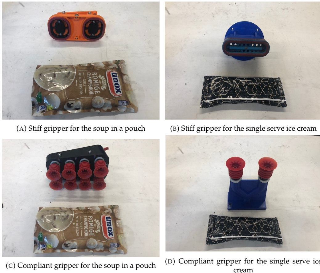
FIGURE 3.3: The four considered grippers and their respective products
