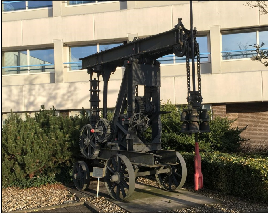
Figure 3.1 photograph of the percussion drill
