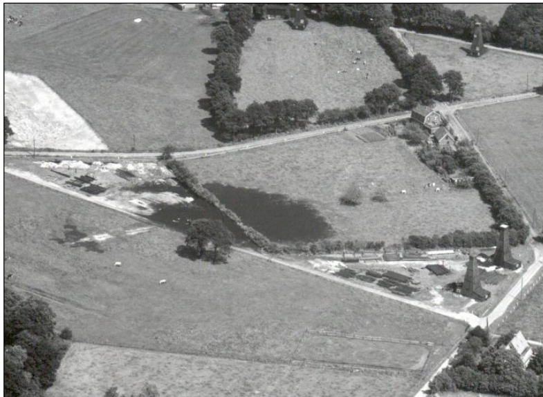
Figure 5.1 Aerial photograph of the water filled subsidence bowl above 18-24, on the right-hand side the wooden derricks of 19 and 20 present (source: AkzoNobel archive)
