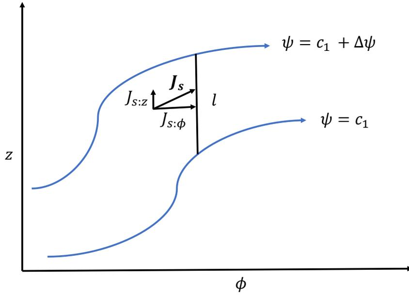
Figure 2.4: Two streamlines and the current density that flows between them.
