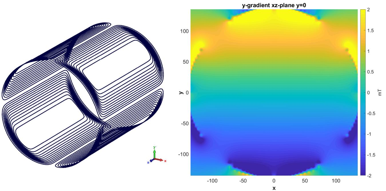
Figure A.6: Left 3D pattern of the y-gradient coil. Right the xy-plane surface plot.
