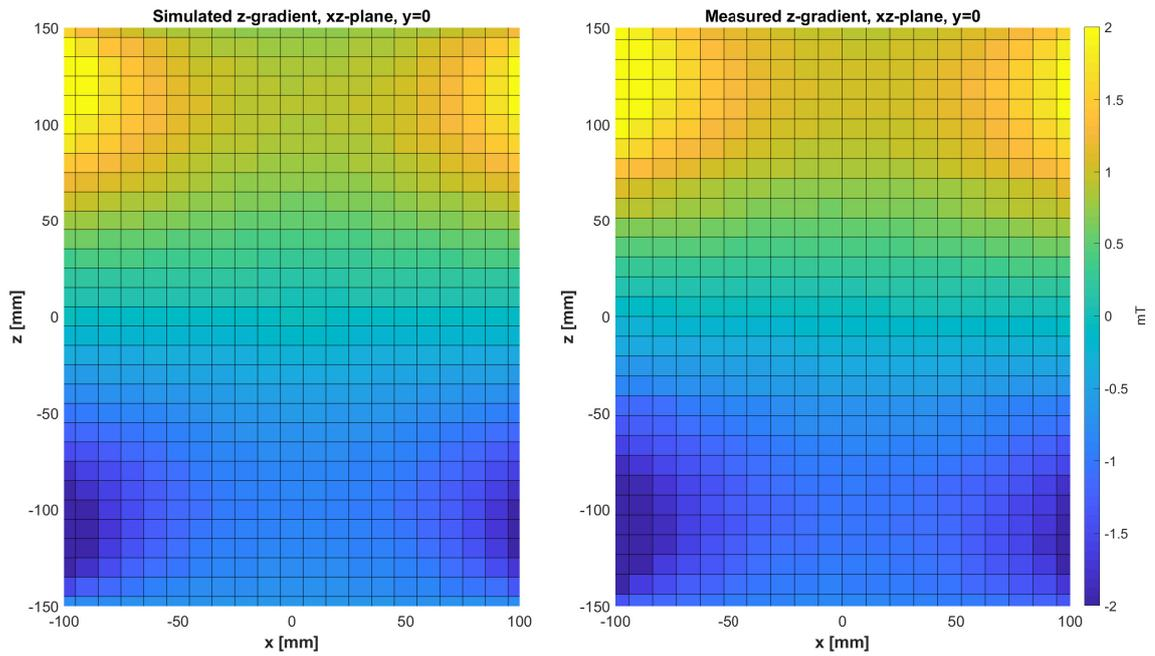
Figure 3.17: Surface plots of the simulated (left) and measured (right) z-gradient coil data. The middle slice of the xz-plane is displayed.
