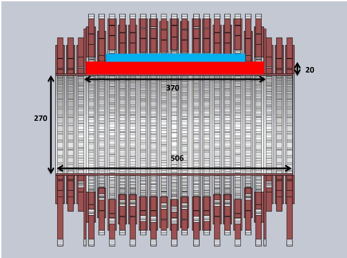
Figure 1.3: Cross section of the low field magnet, the blue rectangle indicates the space where the shim coils are positioned. The red region shows where the gradient coils can be placed this is a region of 370x20mm. All dimensions in the figure are in millimeters. Courtesy of T. O'Reilly (LUMC)
