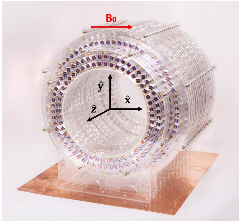
Figure 1.2: The low field magnet system. The system consists of 2948 permanent magnets in a Halbach configuration. The direction of the main magnetic field  $B_0$  is shown with an arrow and is transverse to the bore. Courtesy of T. O'Reilly (LUMC)
