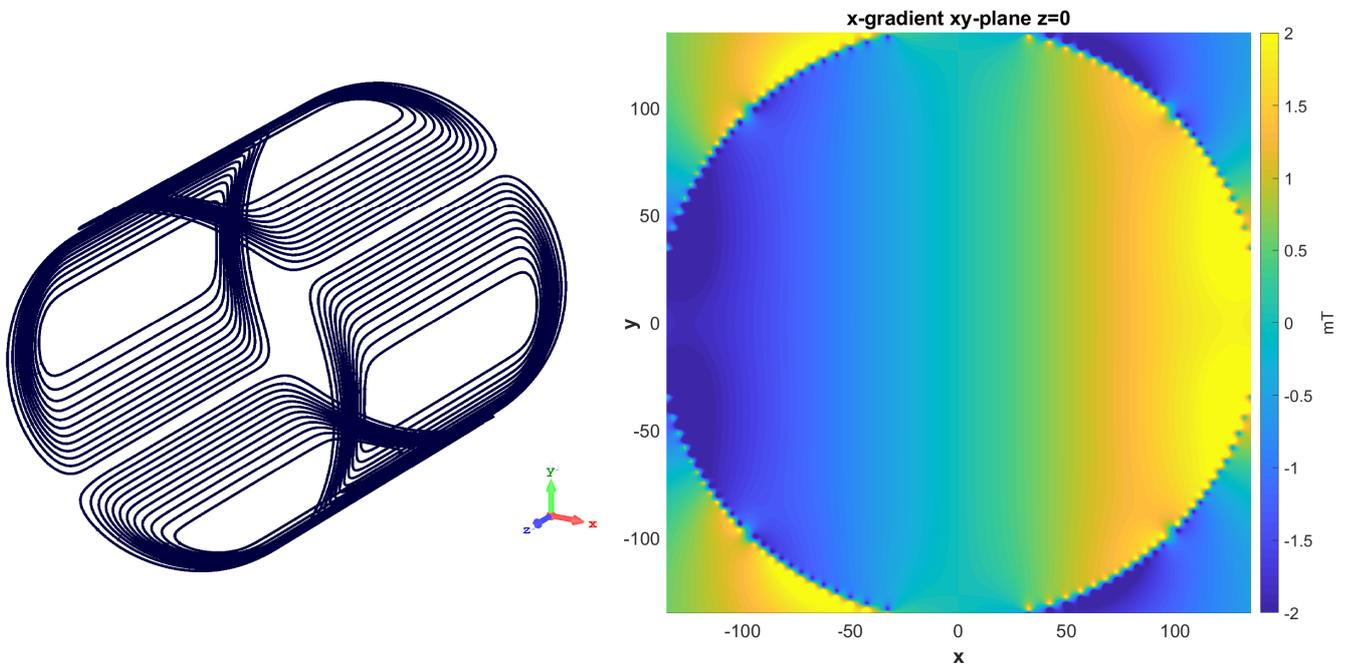
Figure A.2: Left 3D pattern of the x-gradient coil. Right the xy-plane surface plot.
