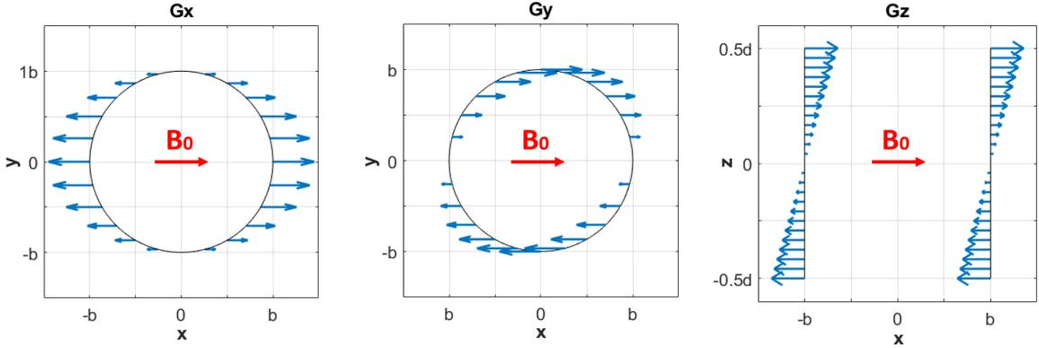
Figure 2.2: Vector plots of the desired gradient fields. From left to right: the x- and y-gradient on a cylinder with radius  $b$  are constant with respect to  $z$ . The z-gradient as seen from a top view, constant with respect to  $\phi$ .
