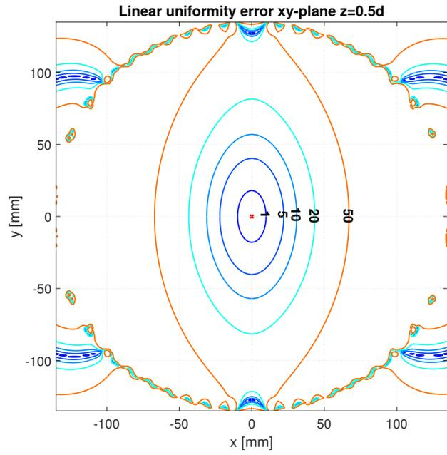
Figure A.11: Left figure shows the linear behavior when taking the values at the middle of the coil along the axis of the bore. This gradient coil is fed with 30[A]. The right figure shows the linear uniformity error of the xy-plane.
