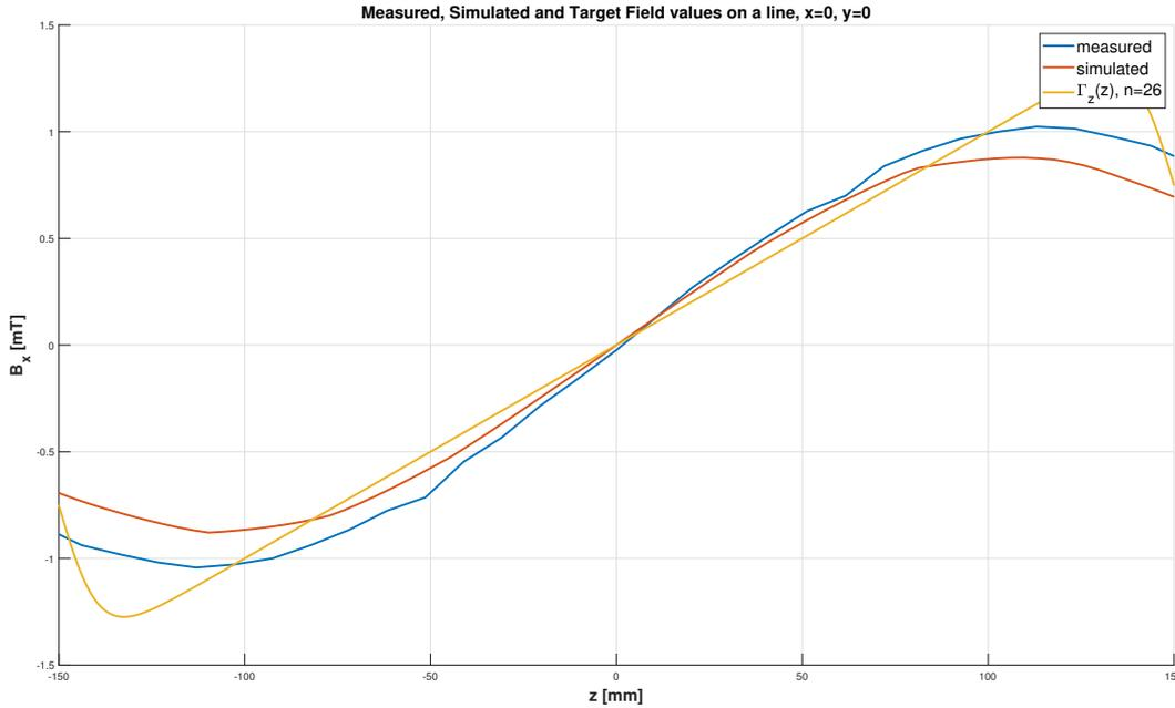
Figure 3.19: Field values on a line through the center of the bore of the measured, simulated and target field. The dips in the measured field at  $z=-50$  and  $z=+60$  are likely to be due to drift in the power supply.
