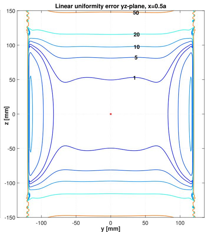
Figure A.4: Linear uniformity error plots of the x-gradient coil. Left corresponds to the xz-plane, right to the yz-plane at  $x=0.5a$ .
