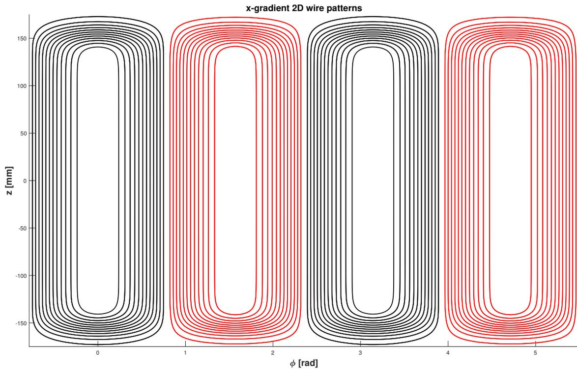
Figure A.1: Two dimensional view of the wire patterns for the x-gradient coil. Red contours correspond to a clockwise direction. Black contours the counterclockwise direction direction.
