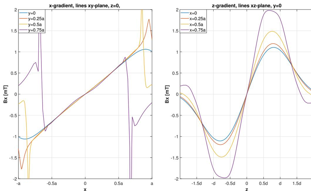
Figure 3.8: Field values taken on lines for the two gradient coils. The lines are taken in the direction of the linear behavior.
