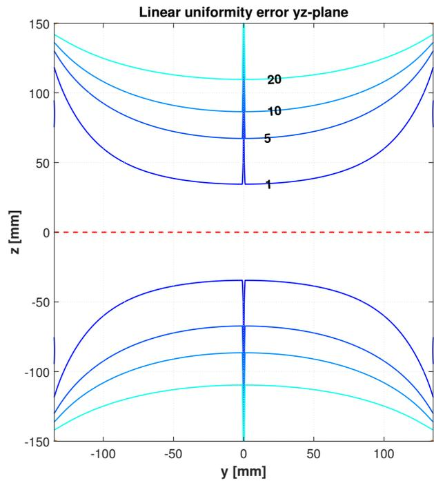
Figure A.8: Linear uniformity error plots of the  $y$ -gradient coil. Left corresponds to the  $xz$ -plane at  $y=0.5a$ , right to the  $yz$ -plane. The error was taken with respect to the red dotted lines.
