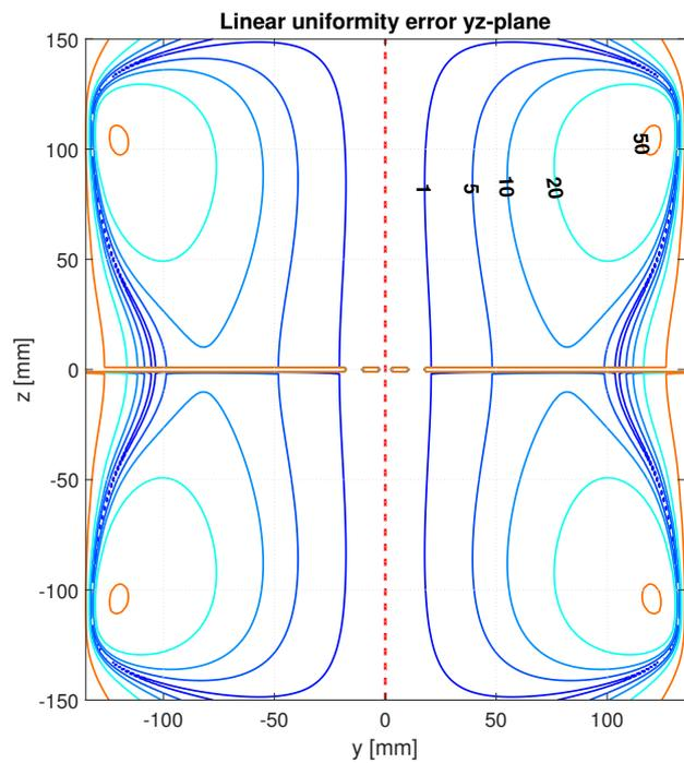
Figure A.12: Linear uniformity error plots of the z-gradient coil. Left corresponds to the xz-plane, right to the yz-plane. The error was taken with respect to the red dotted lines.
