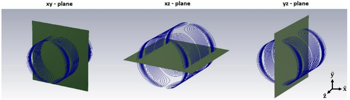
Figure 3.5: The z-gradient coil with the different planes that are distinguished.
