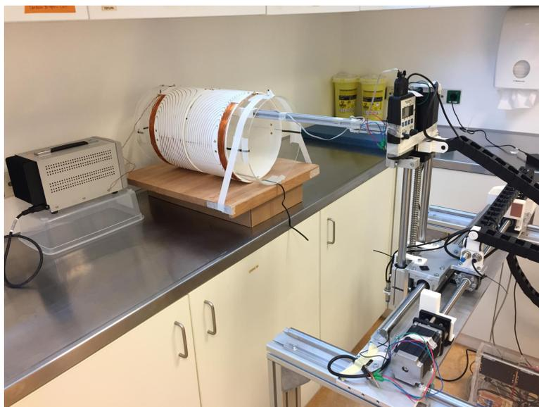
Figure 3.16: The test setup: The gradient coil is fed by the power supply which can be seen on the left. The robot arm with the Gauss-meter moves through the bore of the gradient coil mapping the field.
