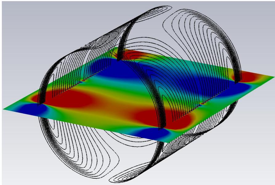
Figure 3.12: The z-gradient coil simulated in CST. This is the coil that is physically built. The intensity plot of the magnetic flux density in the xz-plane is also shown as an illustration.
