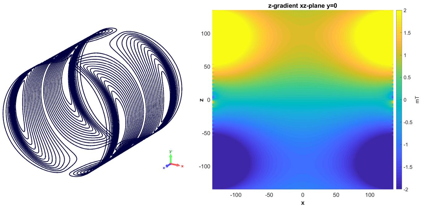
Figure A.10: Left 3D pattern of the z-gradient coil. Right the xz-plane surface plot.
