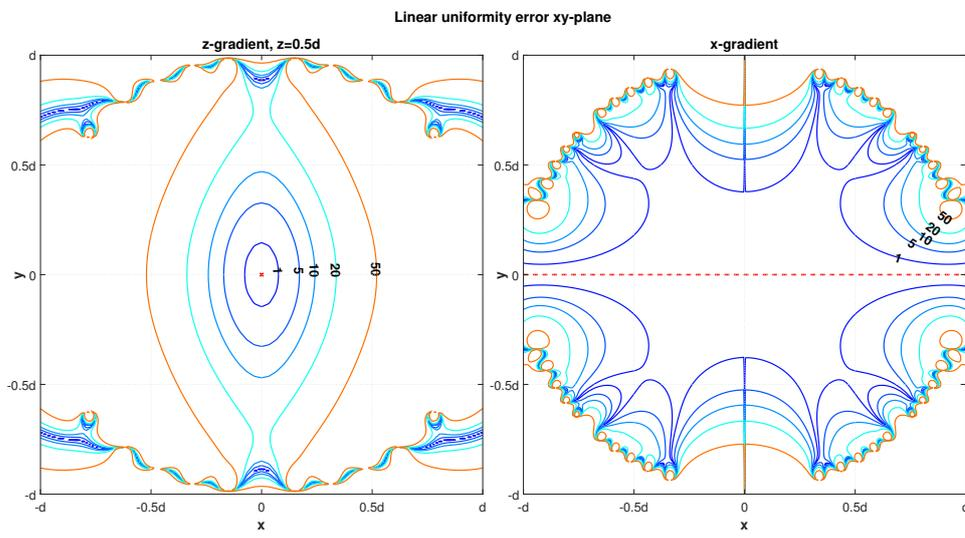
Figure 3.9: Contour plots of the linear uniformity error in the xy-plane. The error is calculated with respect to the central linear line. For the x-gradient this is the line with  $y=0, z=0$ . For the z-gradient the line  $x=0, y=0$  is taken. The red cross or dotted line shows this line. The error is shown in percentage on the contours.
