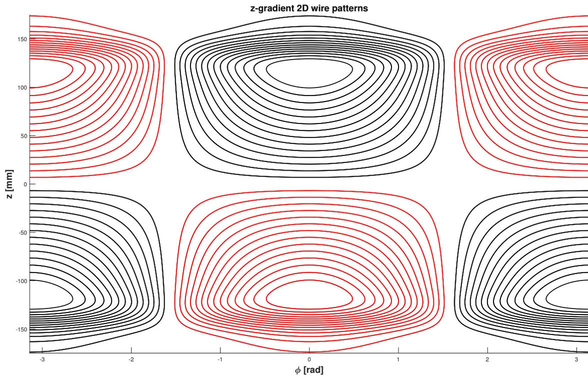
Figure A.9: Two dimensional view of the wire patterns for the z-gradient coil. Red contours correspond to a clockwise direction. Black contours the counterclockwise direction direction.
