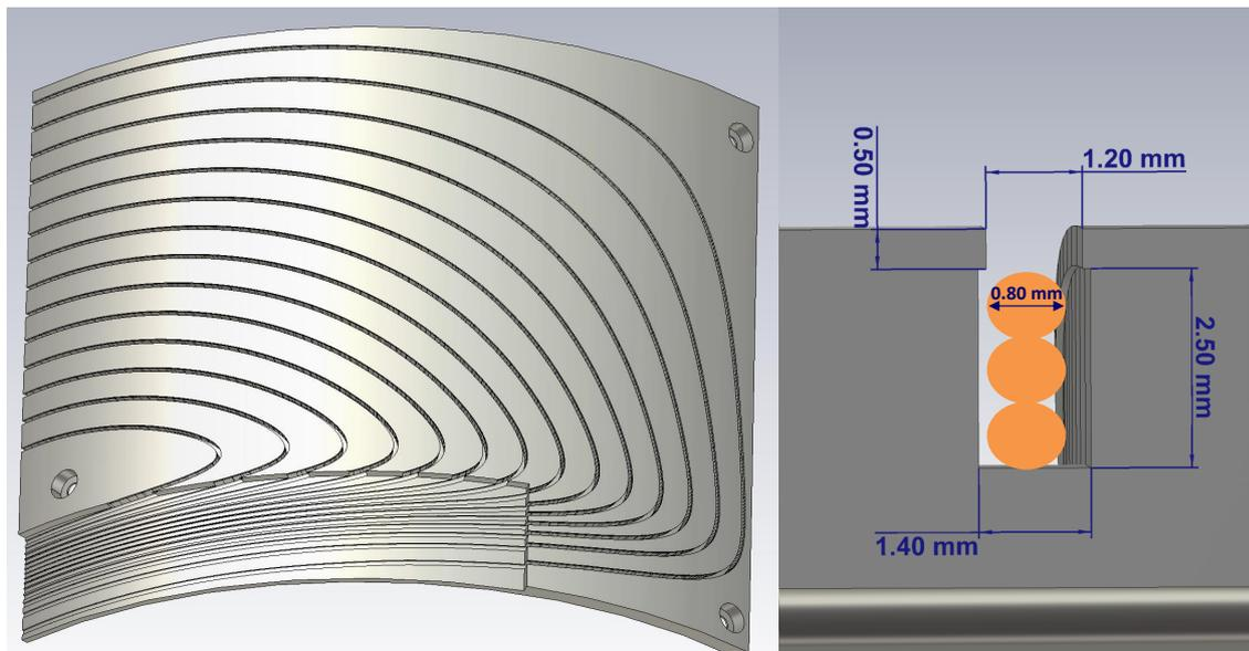
Figure 3.13: The left figure illustrates the schematic of the mold which will hold the wires. This is one eighth of the gradient coil. The right figure shows the profile of the slots which will fit three wires on top of each other. The dimensions of the slot are also given in the figure.
