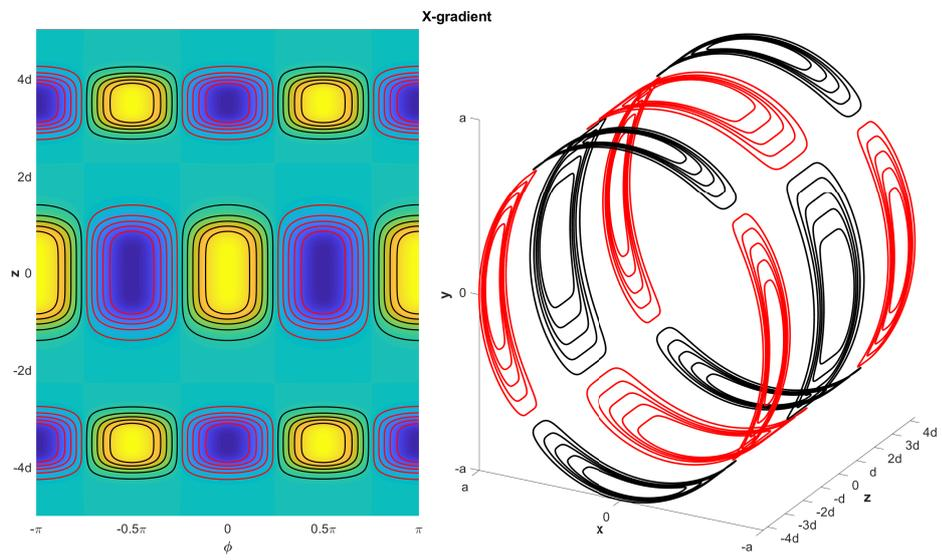
Figure 3.1: The left figure shows the normalized stream function and corresponding current paths of the x-gradient. Yellow corresponds to positive stream function values, blue to negative. The right figure is the 3D representation of the left figure. Black corresponds to counterclockwise red to clockwise.
