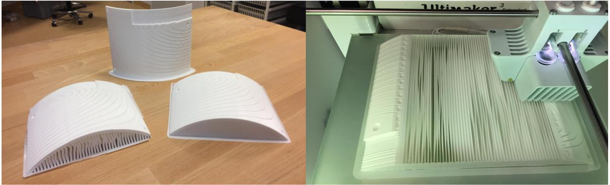
Figure 3.14: The left figure shows the resulting molds created with three types of printing techniques. The mold on the right laying on its back is the one with the best slots. The right figure shows the 3D printing process.
