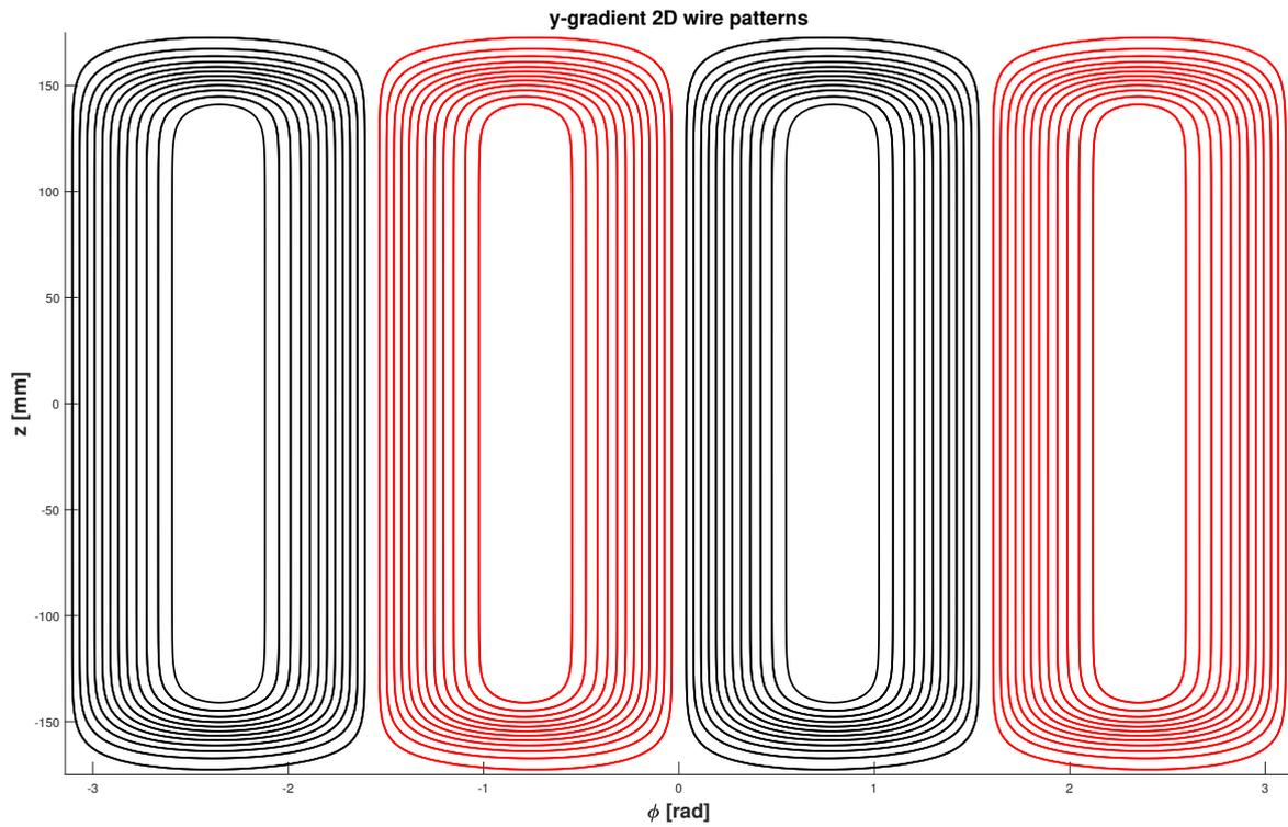
Figure A.5: Two dimensional view of the wire patterns for the y-gradient coil. Red contours correspond to a clockwise direction. Black contours the counterclockwise direction direction.
