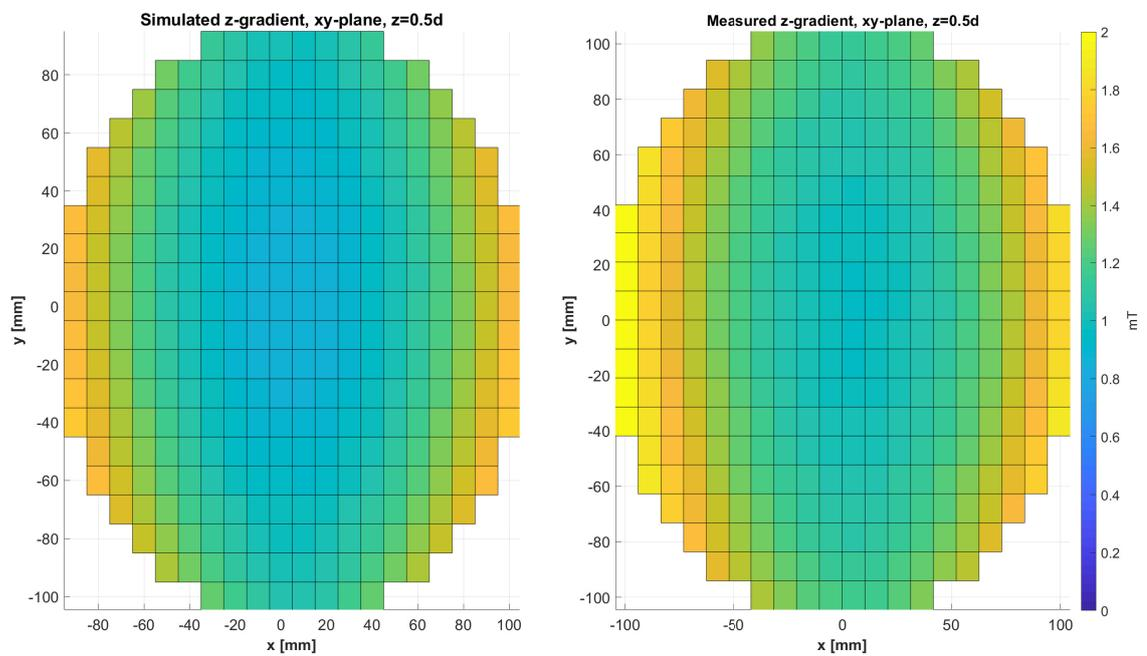
Figure 3.18: Surface plots of the simulated (left) and measured (right) z-gradient coil data. A slice at  $z = 0.5d$  in the xy-plane is displayed.
