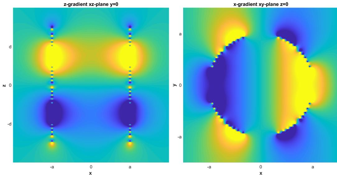
Figure 3.6: CST simulation results for  $z$ -gradient (left), the  $x$ - (right). The figures are intensity plots of the  $x$ -component of the magnetic flux density. Yellow represents positive, blue negative field values.
