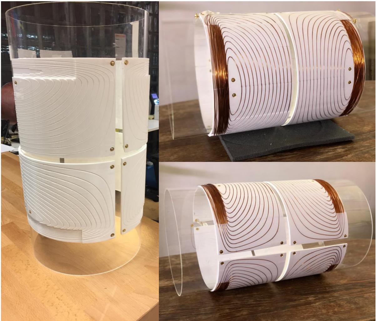
Figure 3.15: the left figure shows the molds mounted on the plexiglas cylinder. The right-hand side figures show the finished z-gradient coil from different angles.
