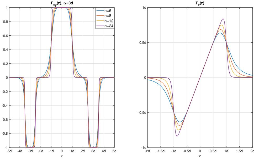
Figure 2.3: The functions used to shape the target fields in the  $z$ -direction for different values of the sharpness parameter  $n$ . On the left the function used for the  $x$ - and  $y$ -gradient, on the right-hand side the function used for the  $z$ -gradient.
