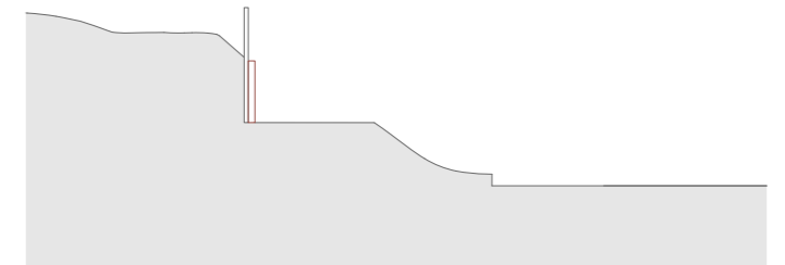
4. In front of this sheet piling, a concrete retaining wall is placed.
