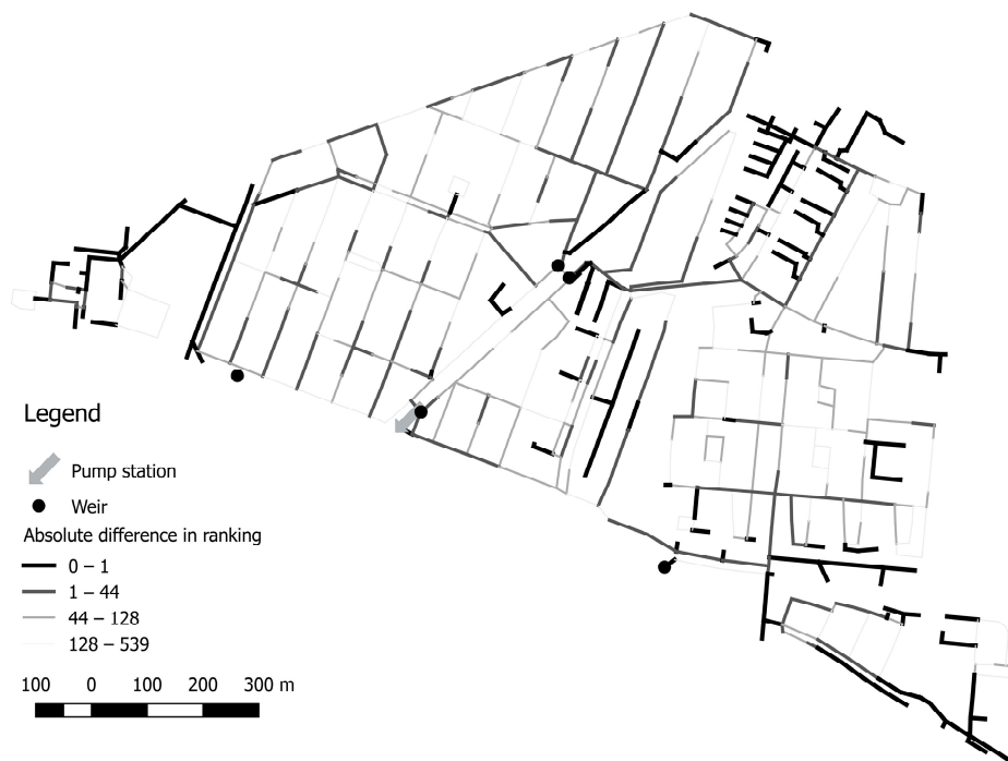
Figure 17. Difference in criticality rank between the HMM and the GTM for Tuindorp. The classification of the groups is based on the equal count method.
