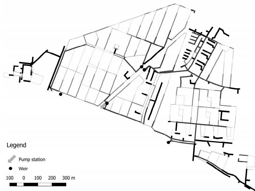
Figure 15. Degree of criticality of Tuindorp: the darker the line, the more critical the conduits.
