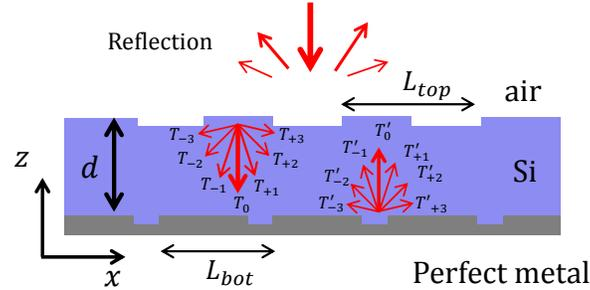
Fig. 9. Light scattering in a double side periodically textured Si-based slab. The periods of top and bottom gratings are indicated as  $L_{top}$  and  $L_{bot}$  respectively. The structure has a thickness  $d$ . The first and second scattering of the incident plane wave inside the structure, is indicated by  $T_i$  and  $T'_i$  respectively. The structure is placed on a grating made of a perfectly reflecting metal. Here, second scattering occurs at the Si-metal interface.
