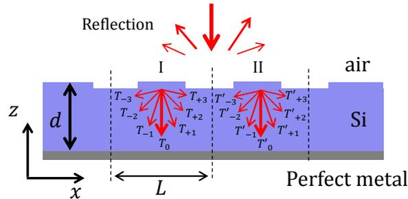
Fig. 1. Light scattering in a Si-based periodically textured structure with thickness  $d$  and period of  $L$ . The two regions, marked I and II, represent the first ( $T_i$ ) and second ( $T'_i$ ) scattering of the incident plane wave inside the structure, respectively. The structure is placed on a flat silver. First and second scattering both occur at Si-air interface
