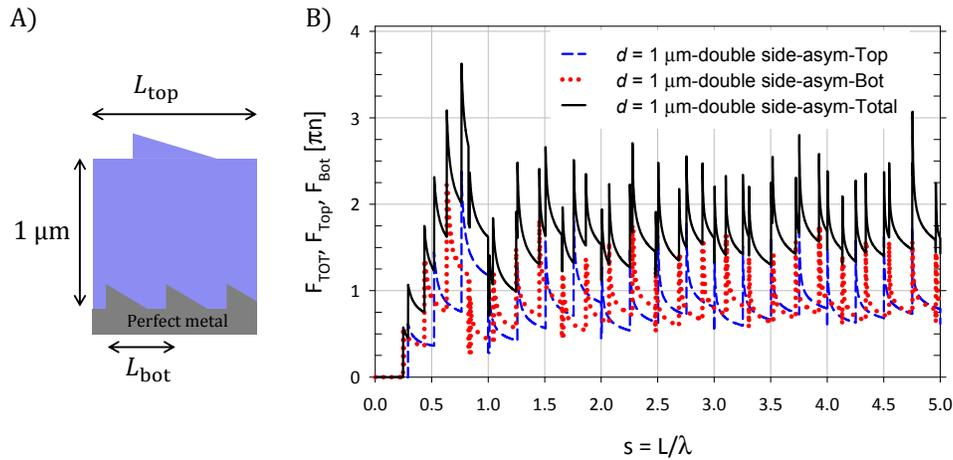
Fig. 11. (A) Schematically shows a 1- $\mu\text{m}$  thick slab endowed with asymmetric grating on two interfaces. The scale of top and bottom grating is exaggerated only for purpose of visualization; (B) reports the absorption enhancement from top (blue) and bottom (red) asymmetric gratings in a 1000-nm thick Si film. The ratio for  $L_{\text{top}} / L_{\text{bot}}$  is equal to 0.909. Total enhancement is shown in black line.
