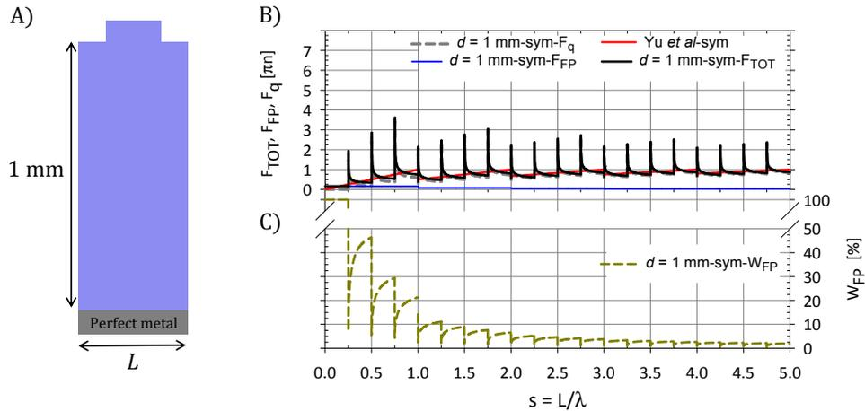
Fig. 4. (A) Schematic presentation of a thick structure with a symmetric grating. (B) Absorption enhancement in a thick Si slab with thickness-to-period ratio  $L/(n \cdot d) = 1.5 \times 10^{-4}$  ( $d = 1 \text{ mm}$ ) endowed with a symmetric grating. (C) represents the  $W_{\text{FP}}$  for the structure shown in (A).
