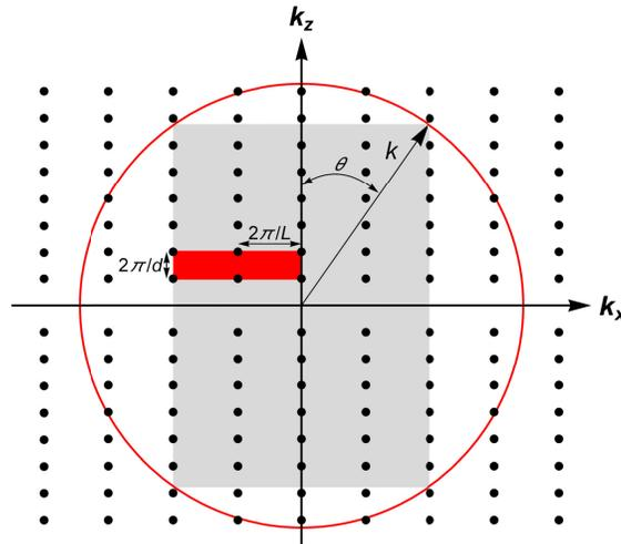
Fig. 2. Resonances (black dots) in a waveguide endowed with a 1-D grating with period  $L$ . The grey region represents the maximum area (in reciprocal  $k$ -space) that can be occupied by all second diffraction orders in the frequency range  $[0, \omega]$ .  $\theta = \arcsin(2 \cdot k_G/k)$  is the angle showing the direction of the  $k$  vector inside the material, when pointing at the highest second order resonance.
