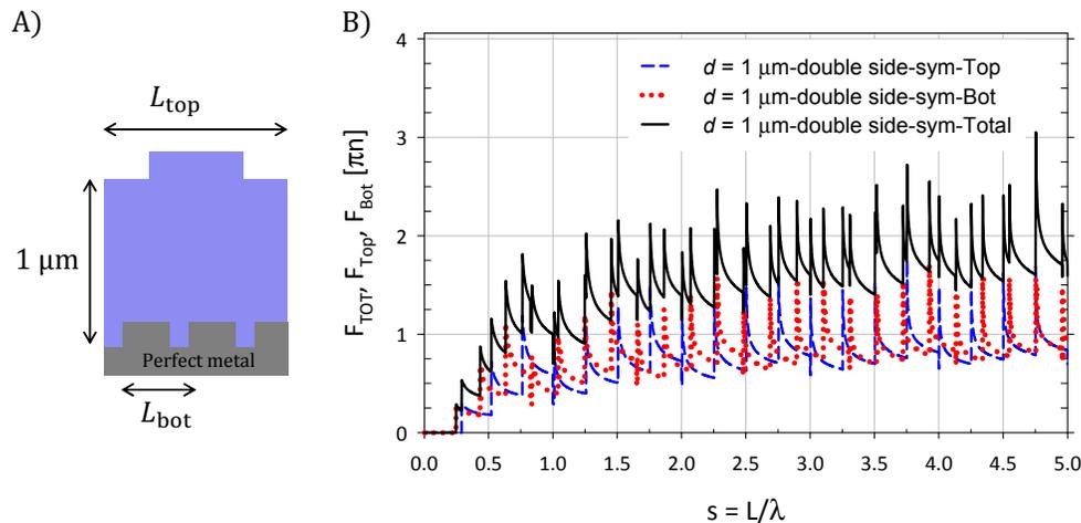
Fig. 10. (A) schematically shows a 1- $\mu\text{m}$  thick slab endowed with symmetric grating on two interfaces. The scale of top and bottom grating is exaggerated only for purpose of visualization; (B) reports the absorption enhancement from top (blue) and bottom (red) symmetric gratings in a 1000-nm thick Si film. The ratio for  $L_{\text{top}}/L_{\text{bot}}$  is equal to 0.909. Total enhancement is shown in black line.
