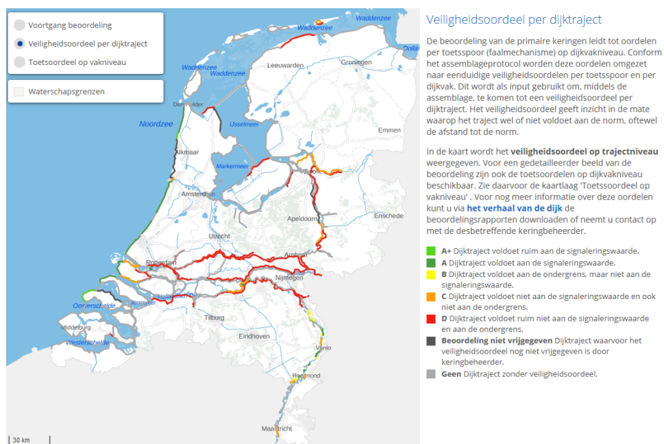
Figure 1.2: Safety assessment per dike segment, status of October 2021. Green and yellow dike segments comply with the safety standards, orange and red do not. Source: Waterveiligheidsportaal (2021)
