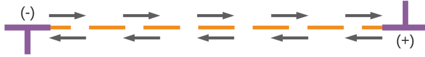
Figure 3.1: Schematic breakdown of a dipole with two 2D edge dislocations in purple and with opposite signs, and the glide plane in 2D as line in orange, defined for a positive \mathbf{b} from left to right. The arrows show the displacement field around the dipole. This convention is used throughout this report.
