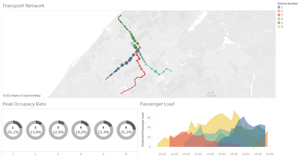
Figure 7.17: Screenshot of the real-time dashboard. It displays the passenger load for active trips over the network on a map, as well as a pie-chart of the peak occupancy rate over the vehicles and area charts with the passenger load over the vehicles for the past trips. The actual vehicle numbers have been replaced by arbitrary numbers.
