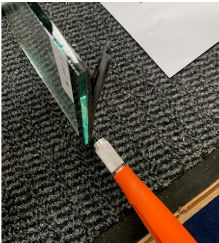
(a) Remove spacer and sealing remain
