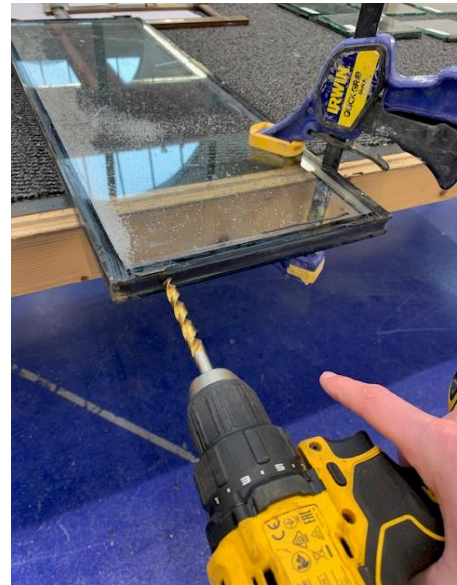
(b) Drill a hole to get between the panels
