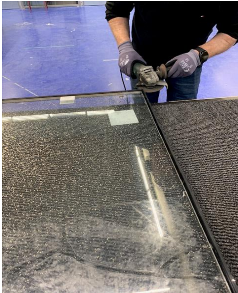
(a) Cut corners with grinder
