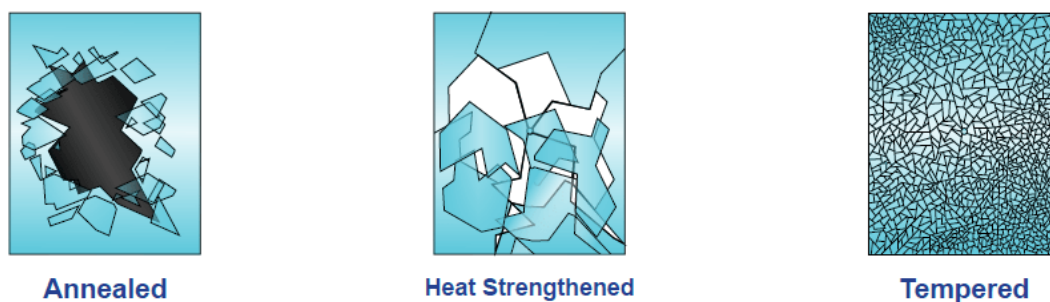
Figure 7. Breakage pattern of different glass types (Peerless Products Inc., 2020).
