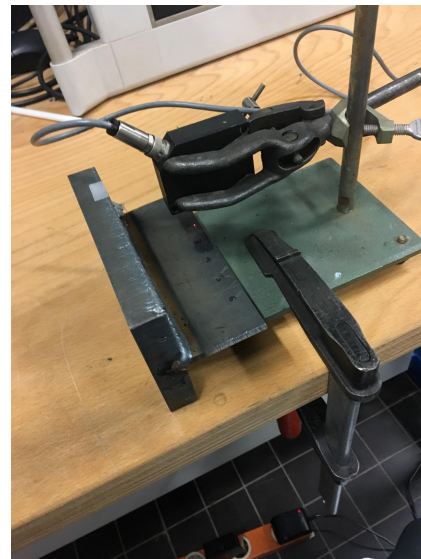
(b) Laser sensor set-up for distortion measurements
