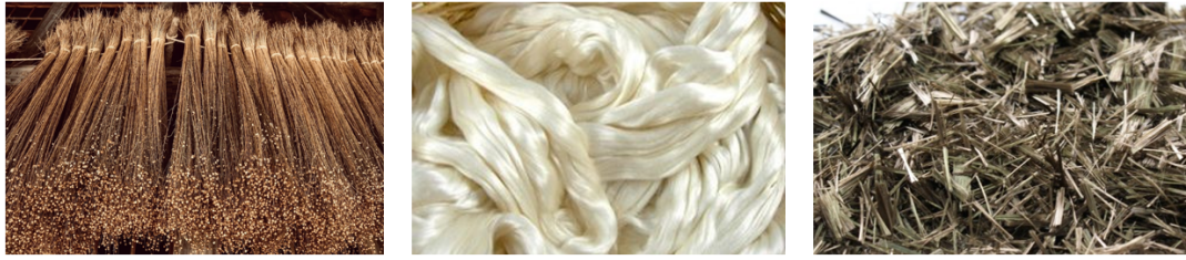
Figure 3.12: Natural fibers: (1) Plant-based flax fiber [41], (2) Animal-based silk fiber [42], and (3) Mineral-based basalt fiber [43]
