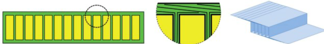
Figure 3.21: Lay-up in sandwich structure using principal of InfraCore [62]
