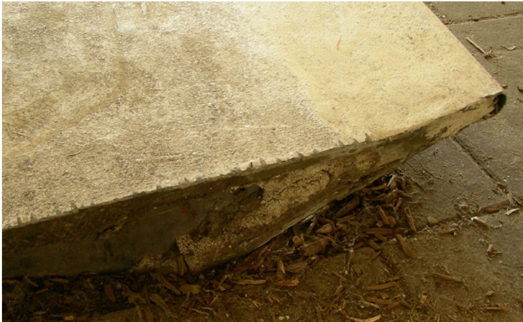
Figure 7. Edge of the rotor blade already brittle with polystyrene coming out, as a consequence of the users walking on it (Photo by Piero Medici, 2011).
