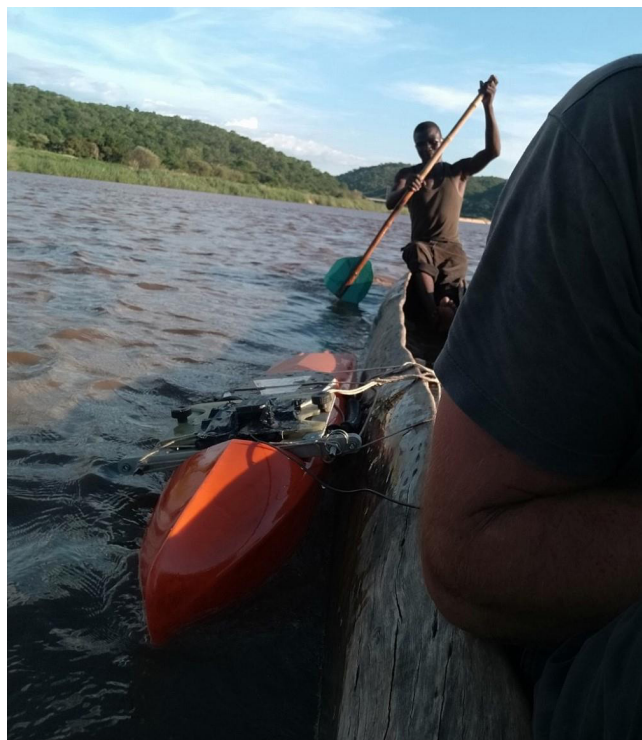
Figure A2. ADCP with a low-cost RTK GNSS attached to a canoe.
