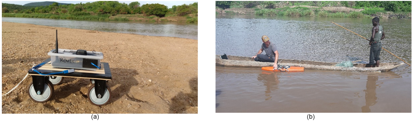
Figure 5. (a) Low-cost RTK GNSS rover mounted on a mobile cart for recording RTK waterline 5 and (b) ADCP combined with an RTK GNSS rover attached to a fisherman's canoe measuring the wet bathymetry.
