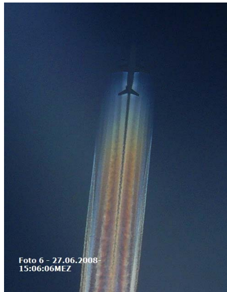
Figure 16. Photograph of an iridescent aerodynamic contrail over Norderney on 27 June 2008, 14:06 UTC [115], with permission from publisher: www.schweizerbart.de .
