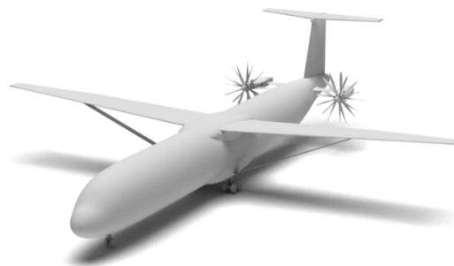
Figure 20. Strut-Braced Wing (SBW) aircraft configuration used in the study; source: DLR-project FrEACs.
