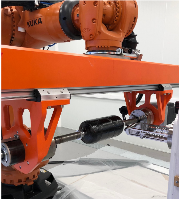
Figure 4.2: Robot-assisted wet winding machinery available at Plastic Omnium.
