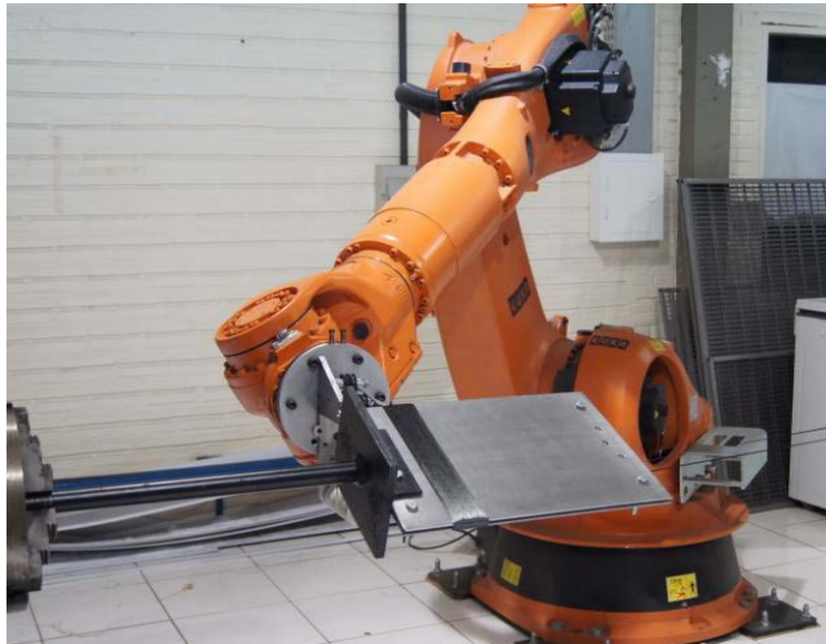
Figure 1.8: Example of manufacturing of unidirectional flat test plates to determine material properties of hoop layers - taken from [61]
