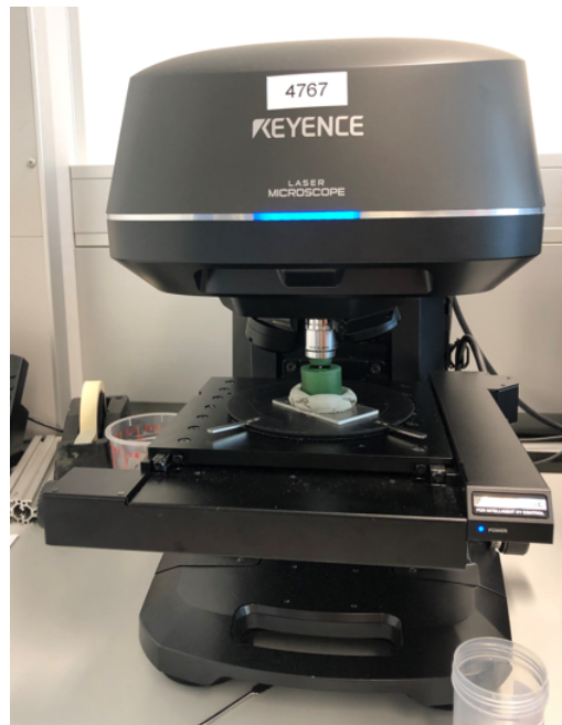
Figure 4.4: Keyence® laser microscope VK-X1000 used for microscope testing.
