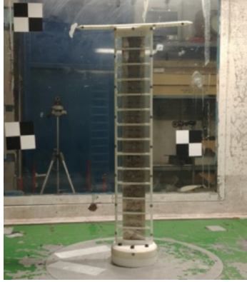
Fig. 1. Pazy wing installed vertically in the wind tunnel test section at the Technion [1]
