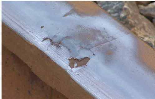
Fig. 5.4. One single squat at a thermite weld with shorter WM (from [15]).
