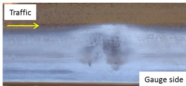
Fig. 1.1. A typical two-lung-like squat where the dark depression, V-shaped crack and the widening of the running band are observed (From Fig. 12 in [9]).
