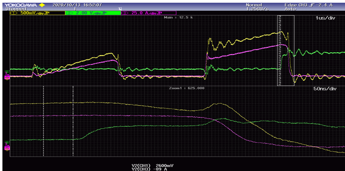
Figure 6.9: Rogowski integrated voltage (yellow curve), current flowing through the switch (purple curve) and comparator output (green curve)
