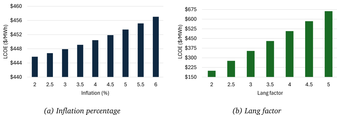
Figure 14: Sensitivity analysis of the a) inflation toward the LCOE; and b) the Lang factor toward the LCOE. The LCOE increases with a higher inflation, although this effect is limited to a maximum of 2.5 percent between an inflation of 2 and 6 percent. The Lang factor has a greater impact on the LCOE, increasing by more than 300 percent with a change in the Lang factor from 2 to 5.
