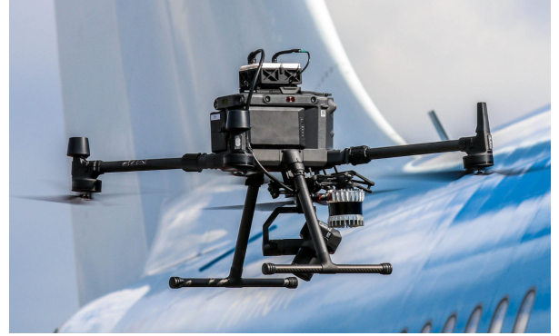
Figure 2. A DJI M300 RTK equipped with a camera, Ouster OS0 lidar and a custom companion computer.
