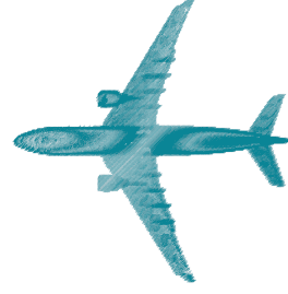
Figure 5. Visualized pointcloud of the casted points of raycasting on an Airbus A330-200 OctoMap.
