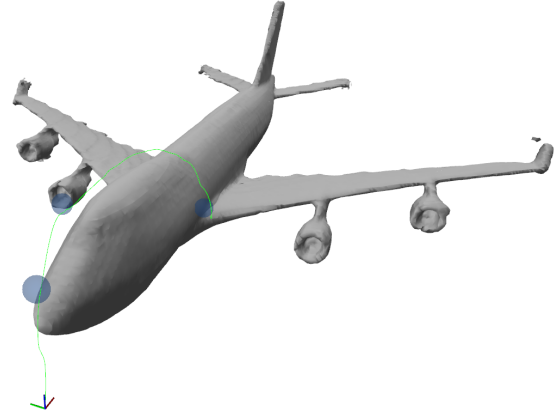
(b) The mesh of a Boeing 747-400F visualized with the waypoints and one of the flown paths (constraint h_2 , \gamma_1 = 2 \text{ s}^{-1} ) under 100 ms delay and no noise.
