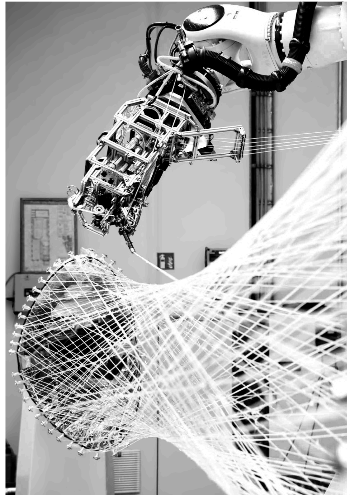
fig.06-01 : cyber-physical robotic coreless filament winding in operation: robotic end-effector winding glass fiber tows
