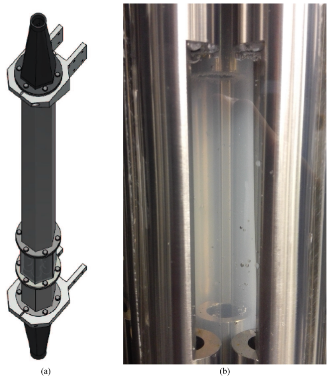
Fig. 2. (a) Overview of the test section. (b) Close-up picture of the silicone rod illustrating the mounting and optical access.
