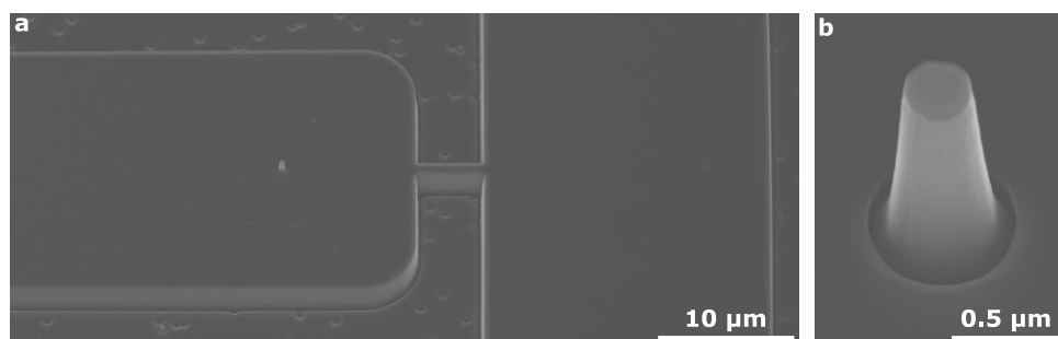
Figure 4.5: Scanning electron microscope (SEM) images of scanning NV probe after etch step II. Taken at a sample tilt of 30^\circ . (a) Scanning probe device. (b) Zoom-in on pillar with a top diameter of 300 nm and a length of approximately 1.5 \mu\text{m} and a tapering angle of about \theta \approx 5^\circ . The HSQ-16 mask is not removed yet.
