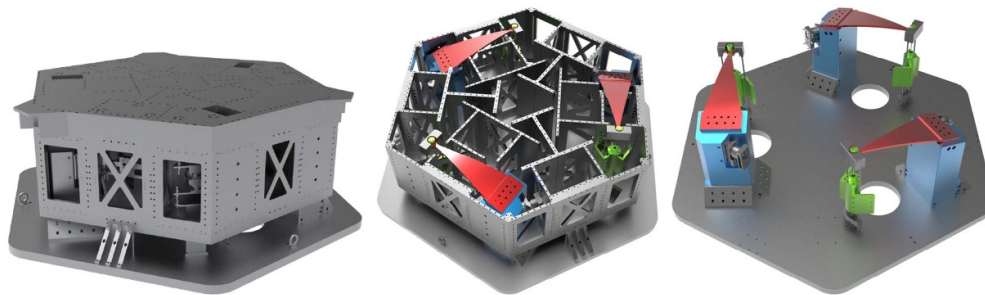
Figure 3. CAD design views of the AP (made of Aluminum). A complete view in the left, an inside view in the middle, and the flexures and blade springs are on the right.
