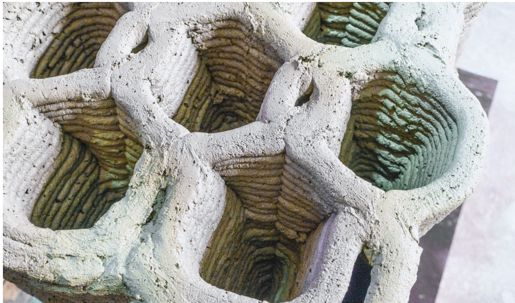
FIG. 1 Close-up of a concrete cellular structure manufactured using extrusion-based 3DCP (Jaugstetter, 2020).
