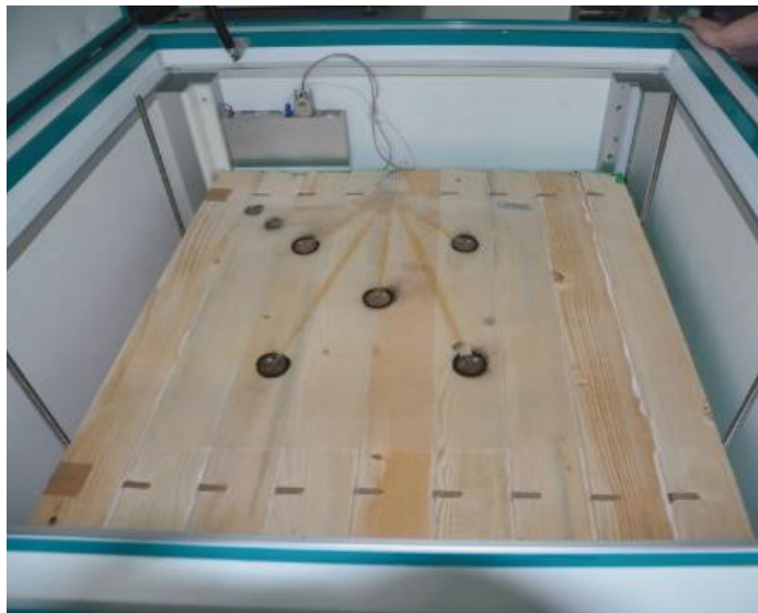
FIG. 6 Hot Box thermal conductivity test
