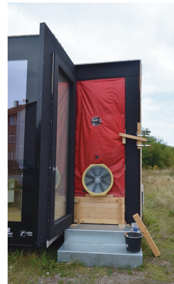
FIG. 7 IBA: Timber Prototype House blower-door test
