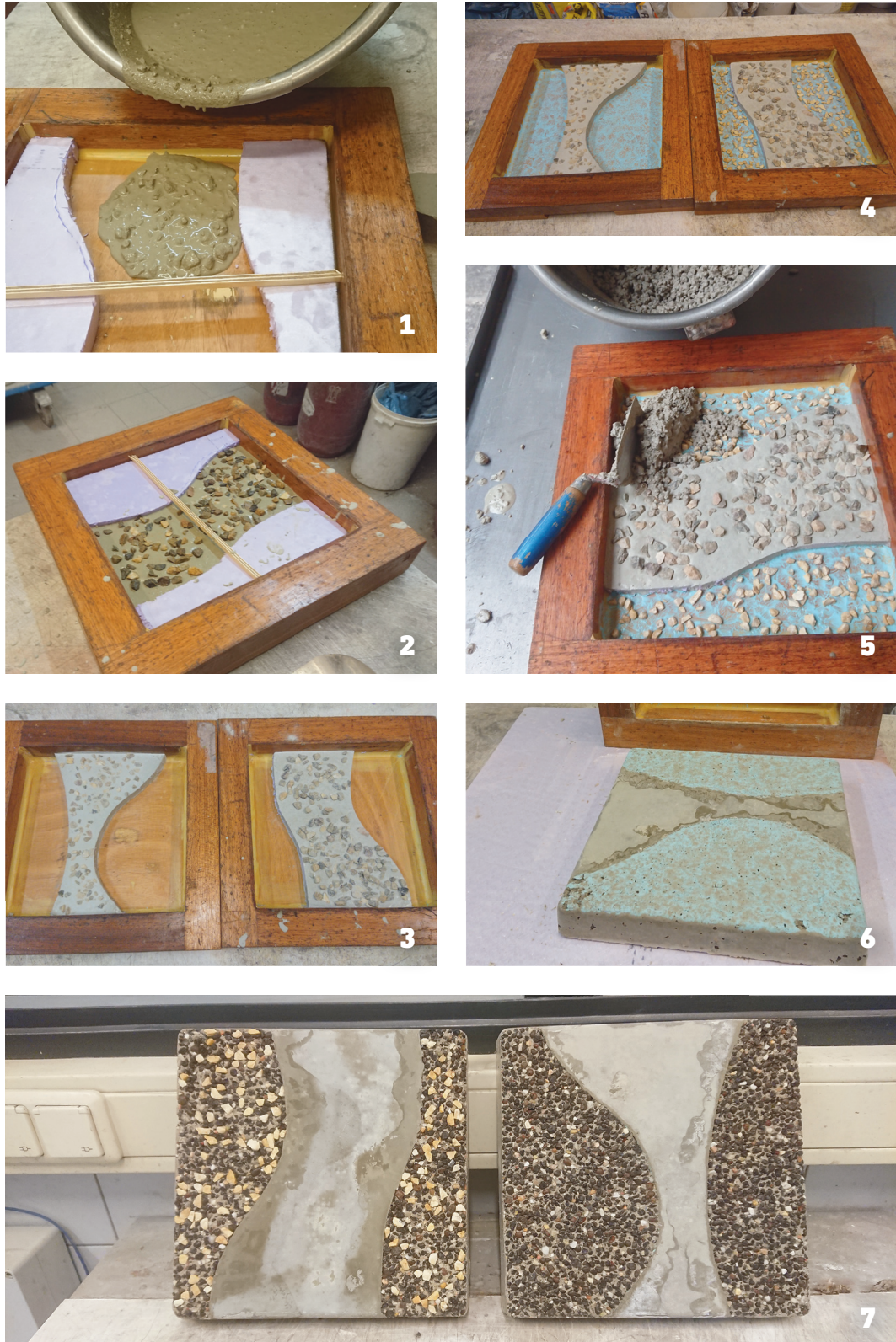
FIG. 4 Overview of the production process of the prototype panels. (1) UHPC concrete is poured into the mould using tempex inserts. (2) Aggregate is added to the top of the UHPC. (3) Tempex inserts are removed. (4) Surface retarder and surface aggregate are added to the bottom of the mould. (5) Bioreceptive concrete is added on to the mould. (6) The panel is demoulded and washed. (7) Final prototype panels.
