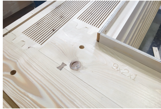
FIG. 11 Assembled corner lap joint detail
