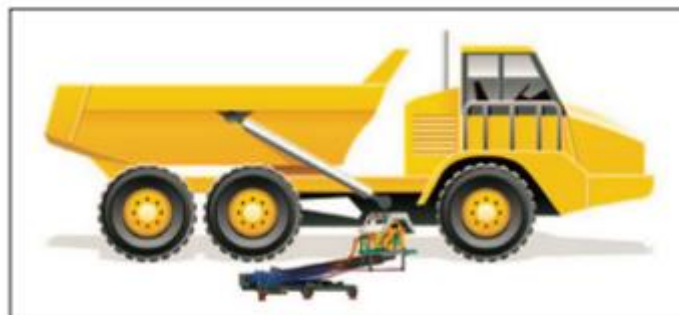
Figure 3.8: Underbody charging method interface (GMG, 2022)
