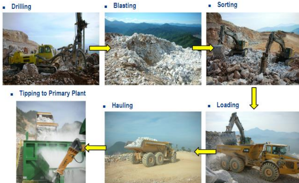
Figure 4.2: Ore mining activities from drilling to crushing
