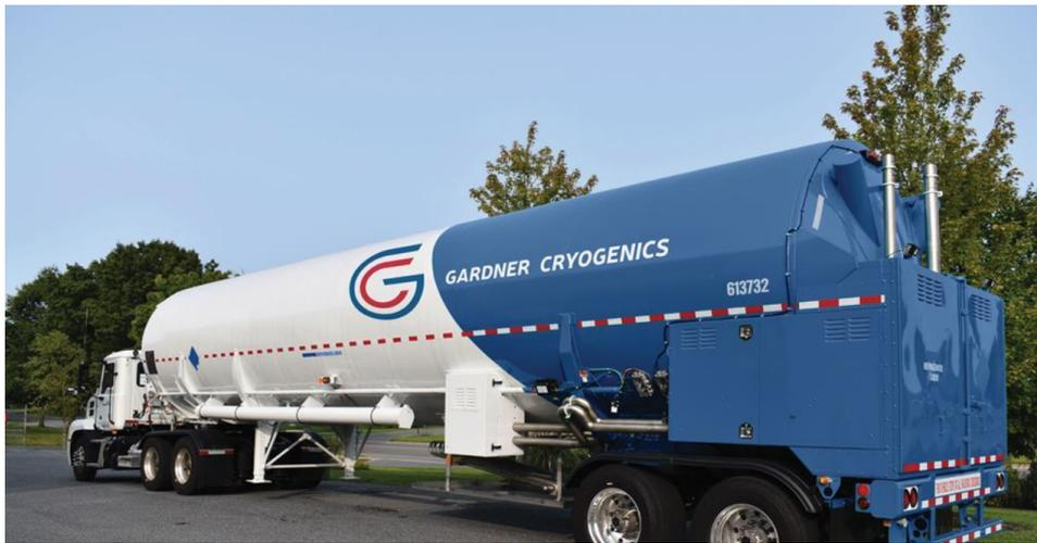
**Figure 4.6:** An example of a Gardner Cryogenics liquid hydrogen tanker [27]
