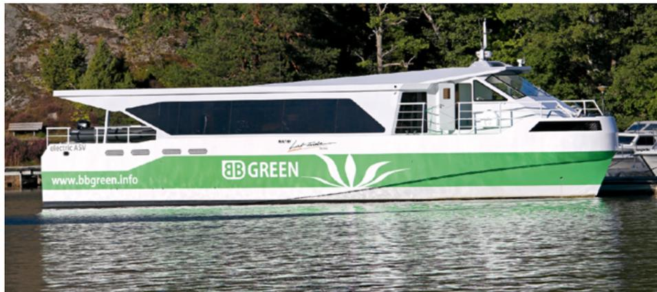
**Figure 4.3:** The BB Green, a fast electric commuter vessel using an LTO Li-ion battery pack [162]
