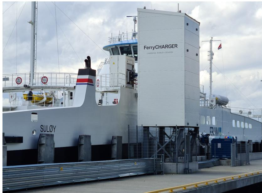
Figure 6.10: The FerryCHARGER used to charge the electric, 400-passenger MF Suløy ferry [57]
