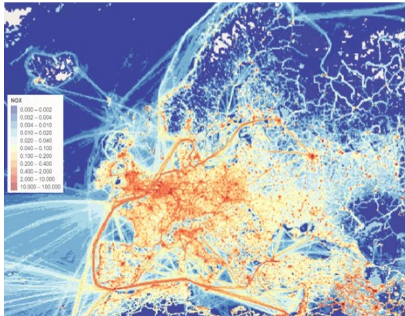
Figure 2.8: NO x emissions from the CAMS-REG inventory for 2017. The total for all sectors is shown. Shipping routes, road networks and large industrial centers are clearly visible. [52]
