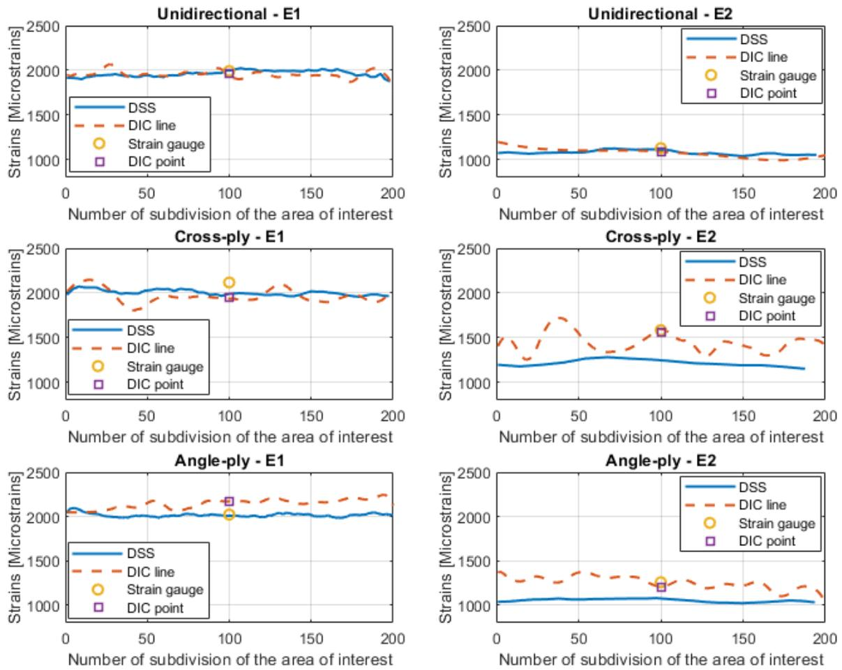
Figure 11. Strain gauge and DSS readings compared to DIC point and line extraction.
