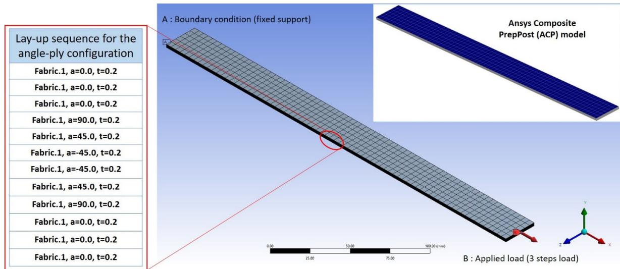
Figure 3. Mesh configuration, boundary condition and applied load.
