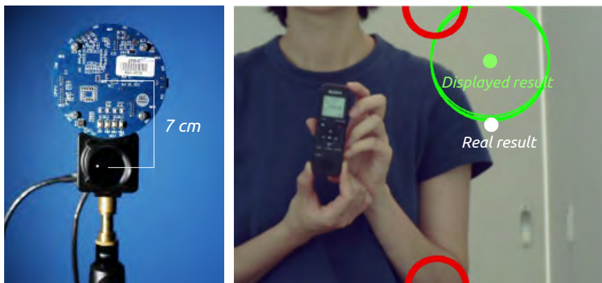
Figure 73 Error caused by the height difference
