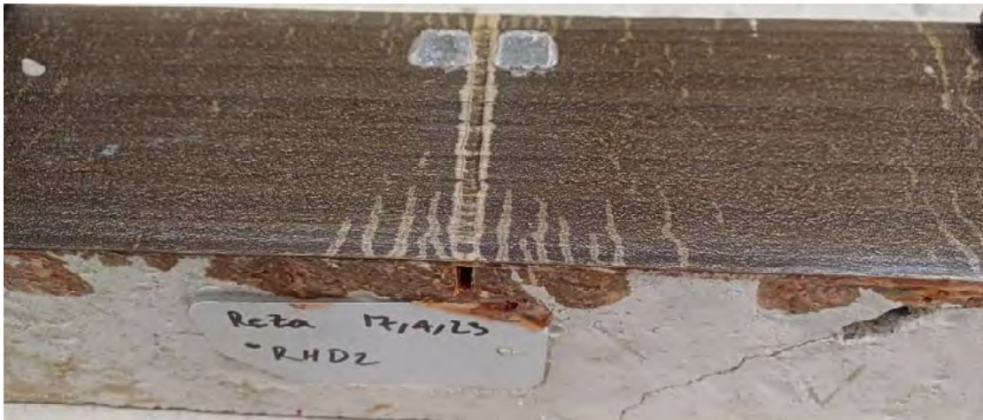
Figure 12. Colour change in the composite of the retrofitted sample, showing the location and size of the developed underneath cracks [19].
