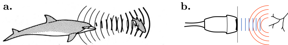
Figure 1-2: The pulse-echo principle is found both in nature and technical applications. The surroundings are perceived by transmitting a pulse and capturing echoes resulting from object interactions. (a) Dolphins apply the pulse-echo principle for echo-location of their prey. Obtained from https://navalunderseamuseum.org (b) In ultrasound imaging the pulse-echo principles is utilized to image internal tissue structures. Lines represent the wavefront.
