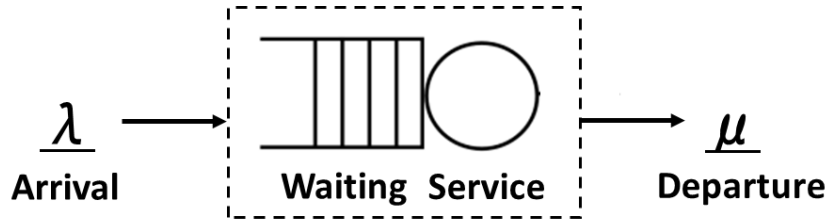
Figure 2.21: Box model of a queueing system (modified from image by Tsaitgaist, by TU Delft – Ports and Waterways is licenced under CC BY-SA 3.0).
