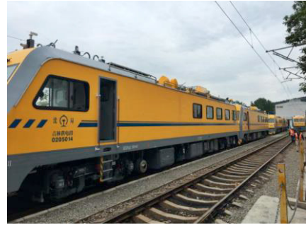
Fig. 2. XLN4C inspection vehicle
